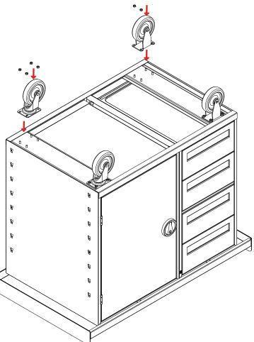
**4.** To operate the caster brakes, press down on the front of the brake with a foot to lock. Then press down on the back of the brake with a foot to unlock.
